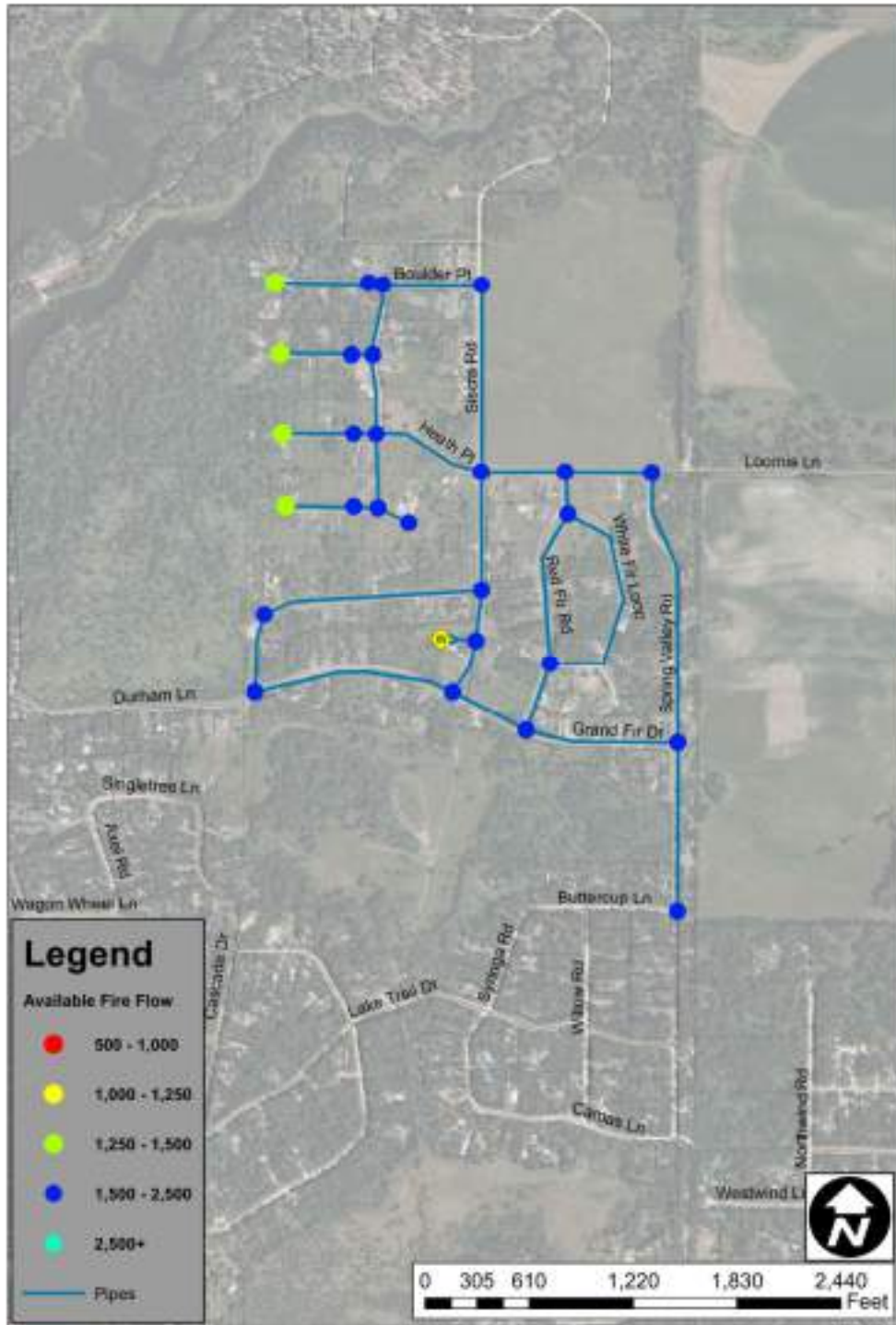
FIGURE 6-15: FIR GROVE EXISTING AFF (BOTH PUMPS)
