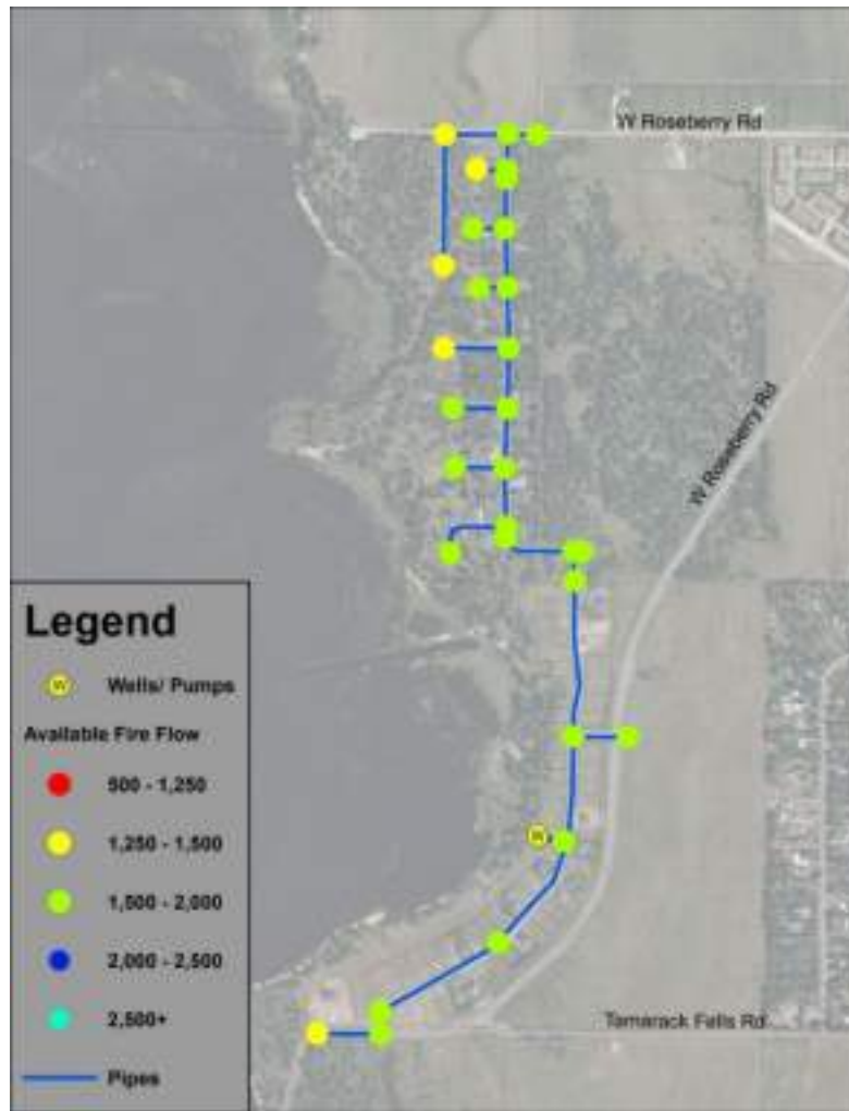
FIGURE 6-11: HAWKS BAY EXISTING AFF (BOTH PUMPS)
